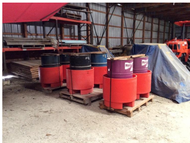
14. Additional 55-gallon drums of petroleum stored in secondary containment units.
